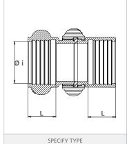
Rocker lug coupling for use with single or double jacket linen hose.
