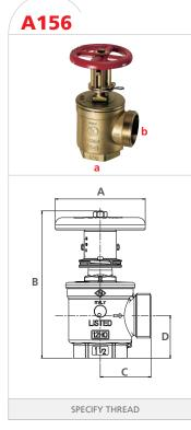
Adjustable restriction of residual pressures up to 175 lb. Locking pin device restricts full opening of valve by untrained personnel, pin may be removed by firefighters to allow full opening of valve.
