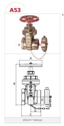
Straightway pattern, non-rising stem, 300 lb. hose gate valves are intended for use on standpipes, fire pumps and hydrants.
