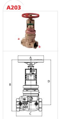
400lb. field adjustable automatic pressure regulating valve for use as a fire hose rack assembly valve or sprinkler control valve where pressure requires regulation.
