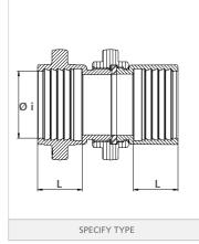
Pin lug coupling for use with single or double jacket linen hose.
