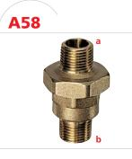
To drain low point of system between swing check valve and Fire Dept. connection. Automatically seals under pressure. Must be installed in vertical position only.
